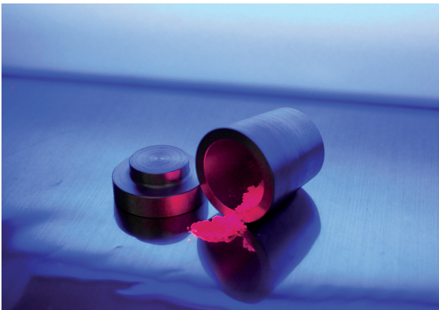
The newly developed phosphor enhances the quality of color rendition by white-emitting LEDs.
